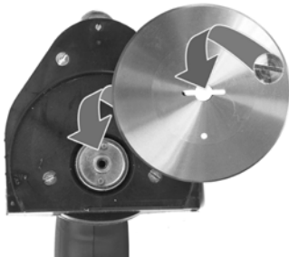
Insert the new knife, screw on the retention disk and fastening screw.
