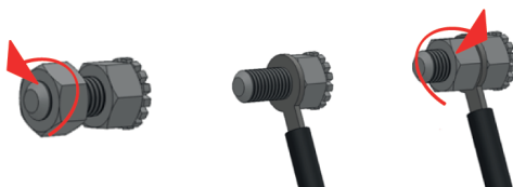
Connection of the device with installation of equalising electrical potentials.
