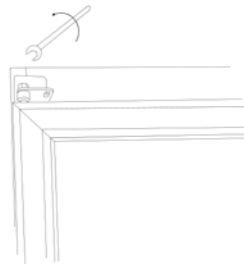
8. Tighten the top hinge pin.
